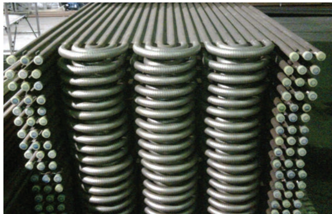
Nappes serpentins de surchauffeur
